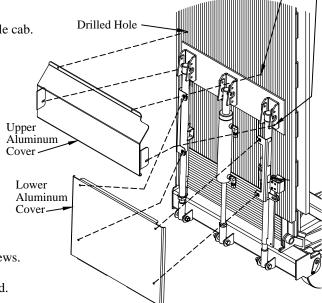
Figure 20: Aluminum cover installation.
