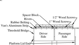
Figure 18: Platform adjustments.
