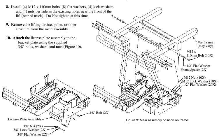
Figure 10: License plate assembly position.
