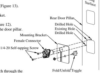
Figure 12: Pendant control female connector location.
