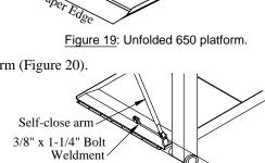
3/8" Flanged Nut — > Figure 20: Self-close arm parts.
