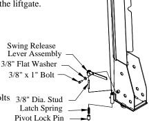
Figure 5: Swing release latch.
