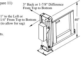
Figure 10: Liftgate properly tipped.
