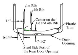
Figure 3: Base plate location and obstructions.
