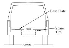
Figure 2: Base plate location and obstructions.
