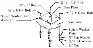
Figure 4: Base plate hardware.
