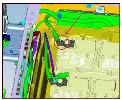
Fig. 1: Location of empty B+ battery post
