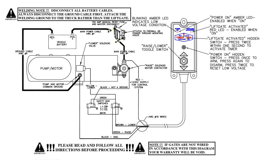
**IMPORTANT:** The pump and motor unit for this lift can require up to 205 Amps of electrical power at 12 volts D.C. Be sure you connect the black cable to the negative terminal of the battery.
