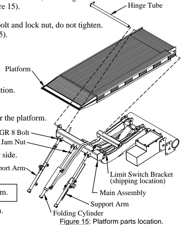
Figure 15: Platform parts location.
