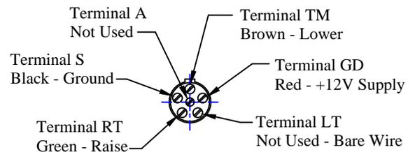
Note: This is a front (terminal end) view, not a rear (wire end) view.
