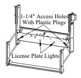
Figure 12: Front access hole location.
