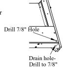
Figure 11: Access hole location.
