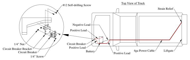
Figure 16: 2019-2023 circuit breaker bracket.
