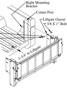
Figure 8: Mounting bracket and liftgate.
