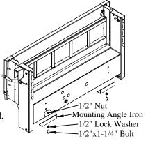
Figure 19: Mounting angle iron location.
