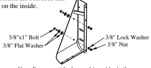
Note: Passenger side shown, driver side similar. Figure 7: Spacer location.
