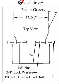
Figure 3: Top view of liftgate bolt-on gussets.
