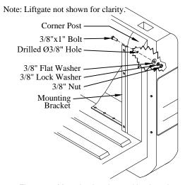
Figure 10: Mounting bracket and backer plates.
