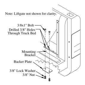
Figure 9: Mounting bracket and backer plates.
