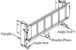
Figure 2: Complete liftgate (62 shown).
