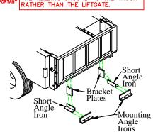
Figure 20: Lower bracket support.
