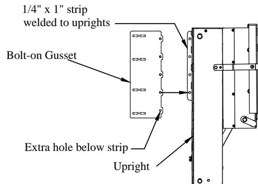
Figure 4: Liftgate requiring bolt-on gussets (**G<sup>2</sup>** shown).
