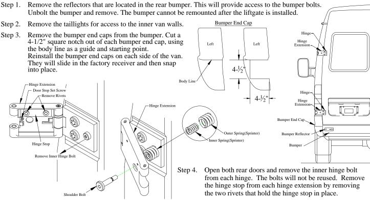
Insert the supplied shoulder bolt through the hole in the hinge extension. Place the inner and outer springs over the shoulder bolt. Push the hinge extension closed aligning the sholder bolt with the threaded hole in the van body. Tighten the shoulder bolt to 20ft-lb with a 5mm allen wrench. Close the doors.
