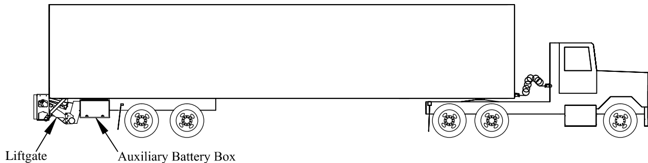
Figure 2: Auxiliary battery box location.
