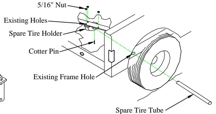
Figure 12: New spare tire holder position.
