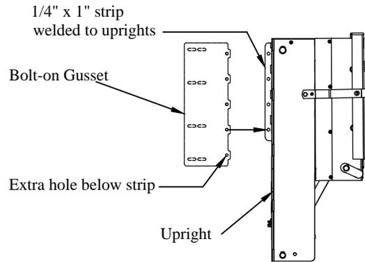
Figure 5: Liftgate requiring bolt-on gussets (G<sup>2</sup> shown).
