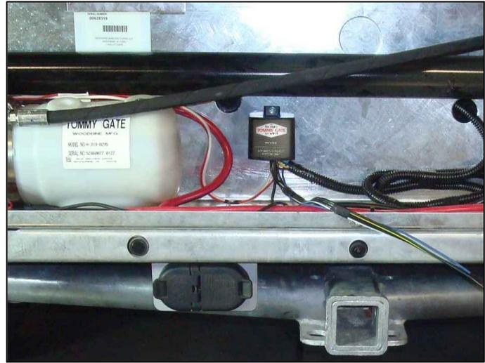
Figure 2: Relay Location (G2 series shown).
