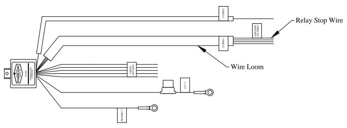
Figure 5: Locating relay stop wire.
