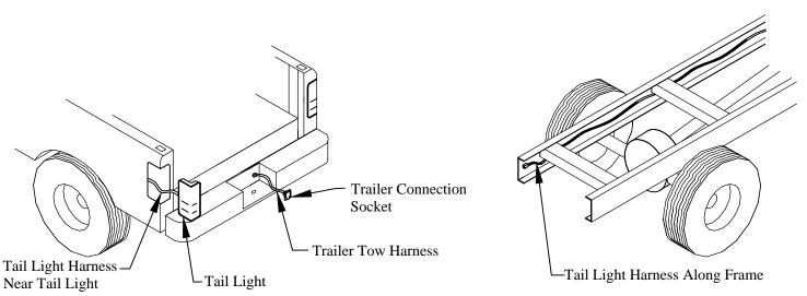
Figure 3: Relay wiring locations (Pickup Box).
