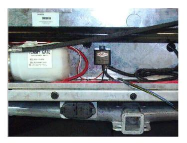
Figure 2: Relay location (G2 series shown).
