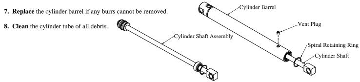
Figure 7: Cylinder disassembly.
