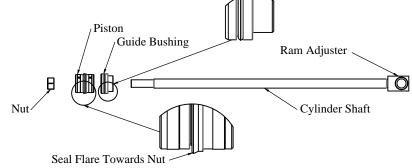
Figure 8: Cylinder shaft assembly.
