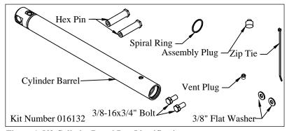
Figure 4: V2 Cylinder Barrel Part Identification
