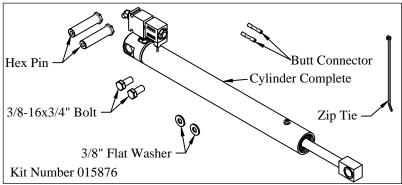
Figure 1: V2 Complete Cylinder Part Identification
