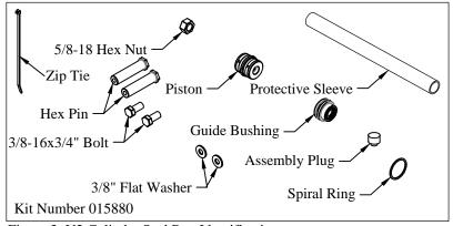
Figure 3: V2 Cylinder Seal Part Identification
