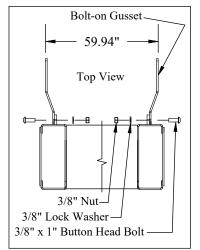
Figure 3: Top view of liftgate bolt-on gussets.
