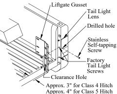
Figure 6: Tail light modification detail (if needed).
