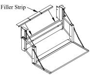
Figure 9: Filler strip placement. Rev 8 4-12-23
