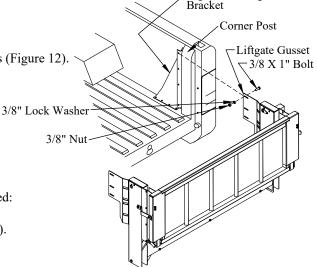
Figure 12: Mounting bracket and liftgate.
