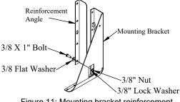
Figure 11: Mounting bracket reinforcement.
