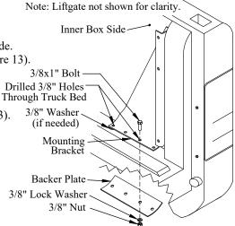
Figure 13: Mounting bracket and backer plate.
