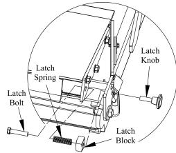
Figure 2: Remove/install latch assembly.
