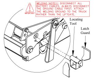
Figure 3: Locate latch guards.
