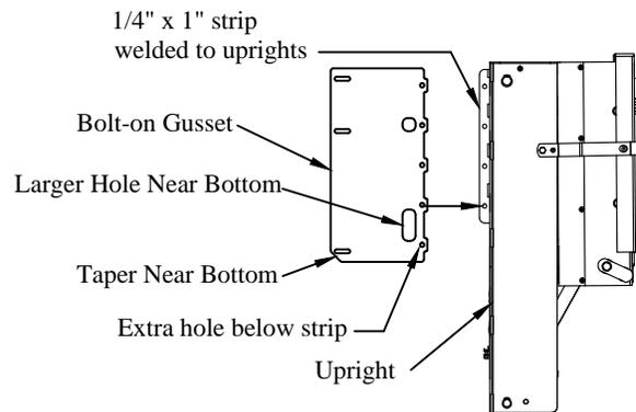
Figure 4: Liftgate requiring bolt-on gussets (G<sup>2</sup> shown).
