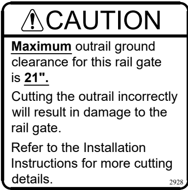
Decal No. 14 Located on the inside of each upright below the mainframe (ABOVE BED GATES ONLY).
