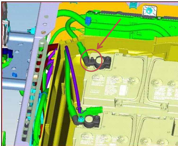
Fig. 1: Location of empty B+ battery post
