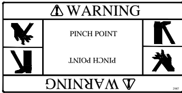
Decal No. 16 Located on smooth side of flipper in the center. (RETENTION RAMP AND RF GATES ONLY).
