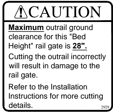
Decal No. 15 Located on the inside of each upright below the mainframe (BED HEIGHT GATES ONLY).
