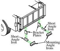
Figure 13: Lower bracket support.
