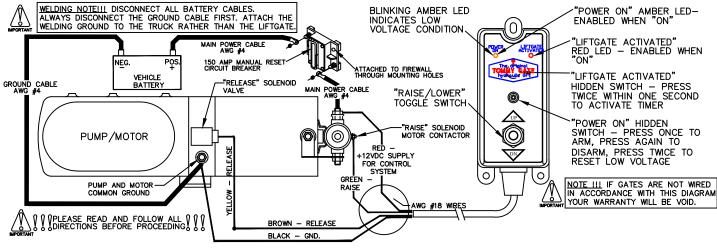
Figure 11: Wiring diagram.
