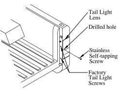
Figure 6: Tail light modification detail.
