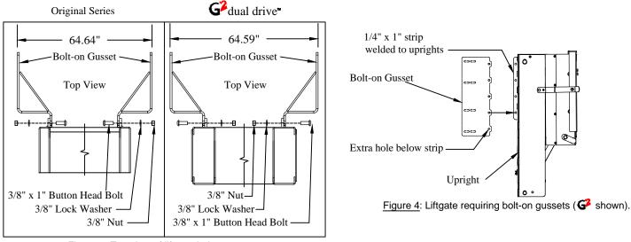
Figure 3: Top view of liftgate bolt-on gussets.
