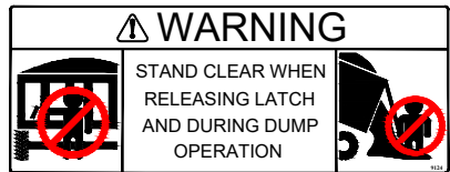
Decal No. 14 Placed on every lift and dump model. Located on the outside top center of the platform
